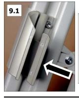
Gently pry open gate hinge sets & fit gate between the inner & outer hinge parts (see Detail 9.1 - 9.5). The "round" posts of the gate will fit through the gap of the hinges (outlined in details above). Secure gate hinges using the remaining  $1/4 \times 3/4$  bolts, washers & nuts. Note that the center holes only require the bolt & nut (no washers will fit). Tighten all hardware & make certain gate opens and closes smoothly.
