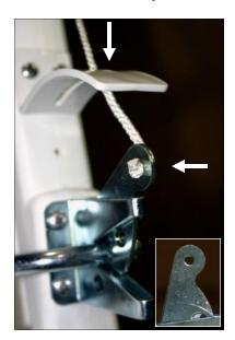
Step 3: Pass end of rope through slot in latch shield and through hole in gate latch. Tie end of rope into a knot so pulling rope will operate gate latch
